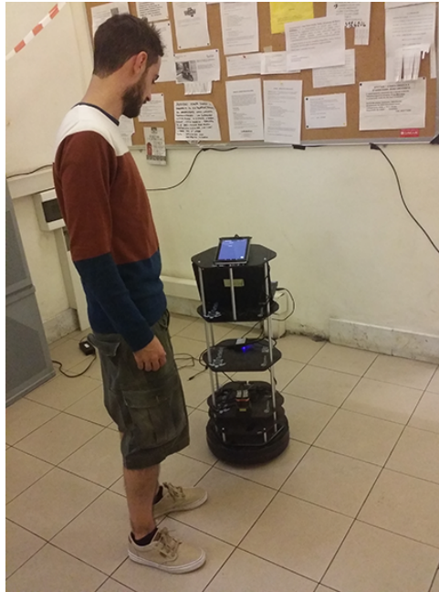
Figure 3.2. Modified TurtleBot robot. The platform deployed is higher than the standard version, and features a tablet which is used to carry out interactions with users.
